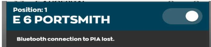
To do this, turn off the vehicle, then pull the main fuse (Located near the battery) for a few seconds the reinstall the fuse and start the vehicle. This will correctly reset the Bluetooth module.
